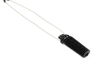
I-T1801.PA-L cable anchor clamp has been designed to ensure the rapid, simple and secure fastening of ADSS fibre optic aerial cables in a range of diameters from 10 to 16 mm. Anchor clamp consists of removable stainless steel bail, UV resistant plastic wedges and body. The automatic, conical tightening system provides no additional tools for installation and considerably reduces assembly time.
